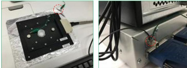
A sheet of aluminum foil serves as an electric shield by grounding. Magnetic field-derived noise cannot be prevented by an electric shield.
