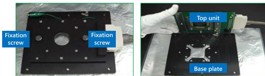
On the base plate, place the MED Probe filled with saline, such as aCSF or PBS holding the ring chamber of the MED probe or the end of the glass substrate. Pay attention so as not to touch the terminals. If any waterdrop, medium or smudge is on the terminal, wipe the terminal with a Kim wipe before setting the MED Probe. Subsequently, place the top unit on the MED Probe and fix with a fixation screw.
