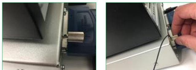
Loosen the screw of the SIGNAL GND terminal, insert the ground wire into the hole (left panel), and fix with a screw (right panel).
